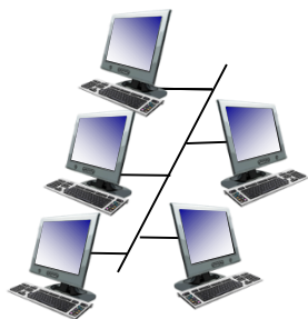
shared wire (e.g., cabled Ethernet)
